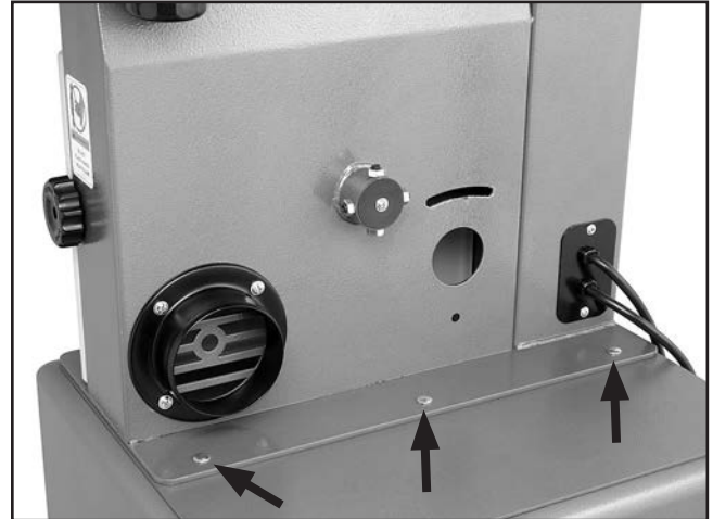
Figure 10. Securing the body to the stand.
